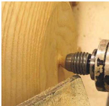
▲ Pic.17 Only put enough tailstock pressure on the work to support and drive it. You should be able to remove nearly all the foot using this fixing
